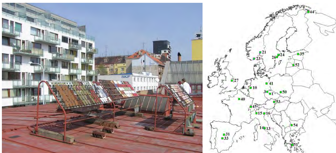
Figure 5: Typical urban test site with materials on a rack (left) and map of test sites (right).
